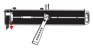
2. Tighten the thumb screws to secure the 4-slot Boomerang in place.
