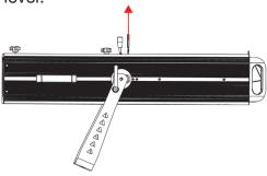
2. Unscrew the retainer screw from the Gobo Holder.
